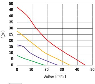
Key Performance curve results are measured at free air, based on the unit running below 19°C and exclude ancillaries
