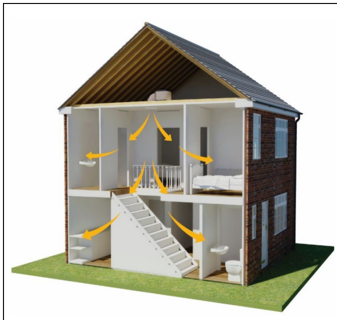
Figure 2 Loft-mounted ventilation unit
