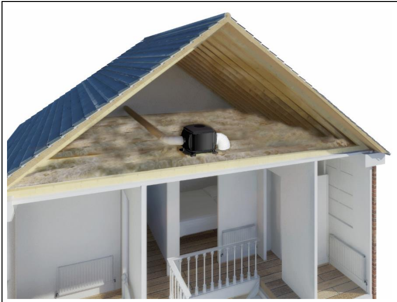
Figure 5 Typical installation of Inline units
