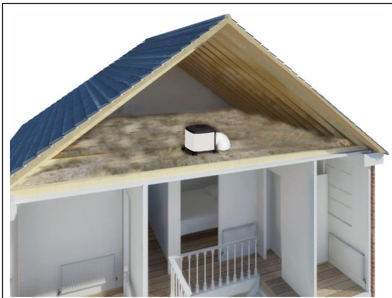
Figure 3 Typical installation of Standard units
