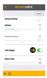
Twin Spigot. For installs where it is necessary to convert a Single spigot unit to a Twin spigot unit, toggle ON. Installer mode only.
