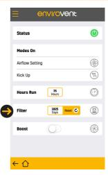
Filter counter shows the current number of days left before the filter needs to be checked. To reset the counter press the Reset button.
