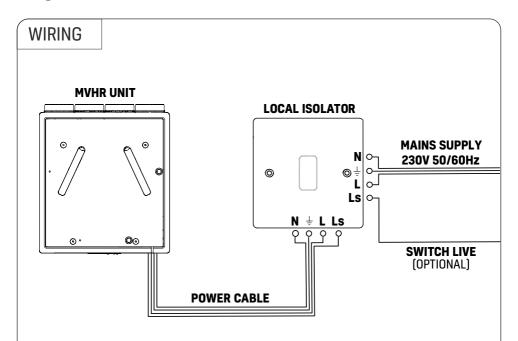
The local isolator must be connected to the mains as part of the fixed wiring. Connect the cores of the power cable to the matching terminals on the local isolator [3A fuse spur or similar].
