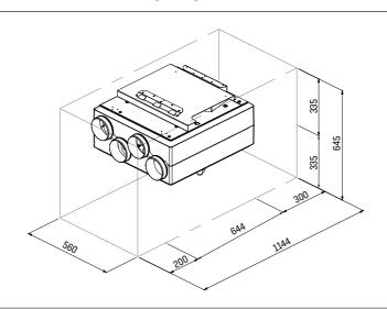
The energiSava® 200 spigots are compatible with ø125mm duct.
