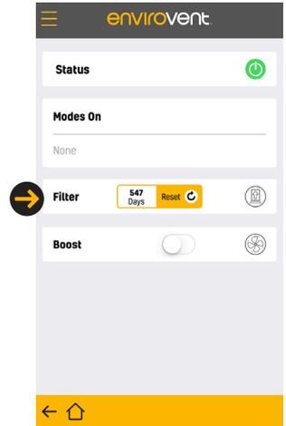
Filter counter shows the current number of days left before the filter needs to be checked. To reset the counter press the Reset button.
