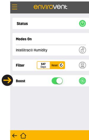
To put the unit into Boost, slide the Boost toggle to the ON position. The Boost run on time is set on the Setting Page. Boost can be turned off at any time.
