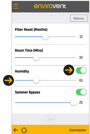
Humidity can be set to 55, 65, 75 and 85%. Factory default is 65%. In installer mode only, humidity can be deactivated. Press **Save** to confirm changes.
