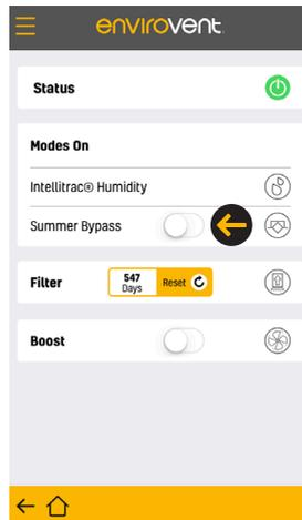
If the bypass is set to MANUAL a Bypass slider appears on the STATUS page. The Bypass can then be turned ON/OFF as required. Default is OFF.
