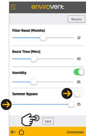
Bypass can be set to 19, 21, 23, 25°C and also set to MANUAL using the slider. Factory default is 25°C with the slider set to AUTO. Press **Save** to confirm changes.
