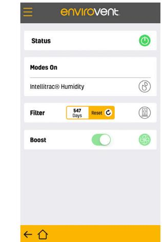
Boost 'ON' is indicated by a green toggle. Note- if the unit is in Switch Boost (i.e. unit boost is wired to a light switch), Boost will show as ON, but greyed out and can't be turned off in the app.
