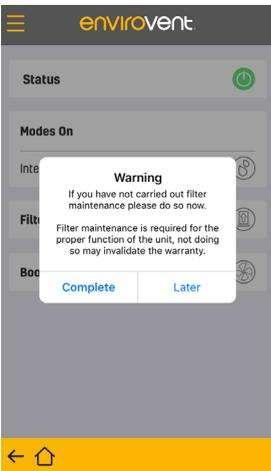
If Reset is pressed a popup appears giving two options. It is important that the filter maintenance is carried out before 'Complete' is pressed.
