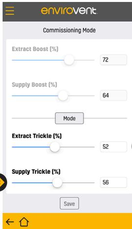
Set Trickle Extract and Supply in the same way as Boost, using the slider or by inputting the figure required.
