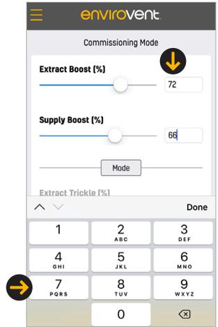
You can also set Boost by pressing on the current airflow figure and inputting a new amount using a key pad. Press 'Done' when complete.
