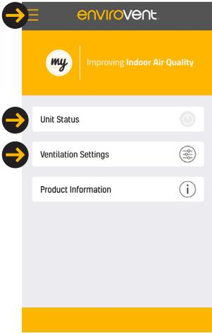
From the Home screen press the Status or Settings tab to start the connection wizard. Alternatively, press 'Connect To Unit' in the drop down menu.
