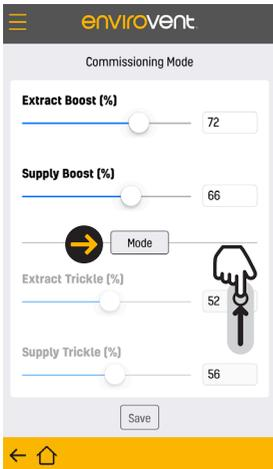
To toggle between Boost and Trickle press the 'Mode' button. On smaller devices pull up on the screen to display the lower half of the screen.
