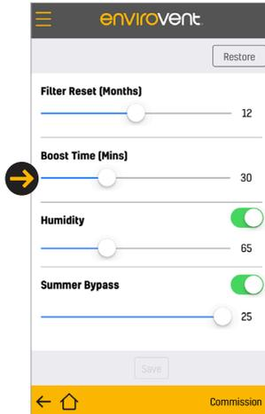
Boost can be set to 15, 30, 45, 60 minutes. Factory default is 30mins. When changes are complete press **Save**.
