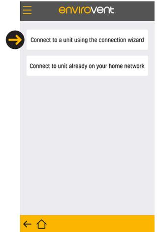
Press the first tab, 'Connect to a unit using the connection wizard'.
