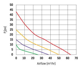
Key Performance curve results are measured at free air, based on the unit running below 19°C and exclude ancillaries
